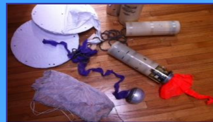
Dismantled sonobuoy. Red bag inflates upon deployment. Electronics package is attached to bag. Silver orb contains DIFAR/hydrophone sensors. White discs used to dampen 'strumming'.
